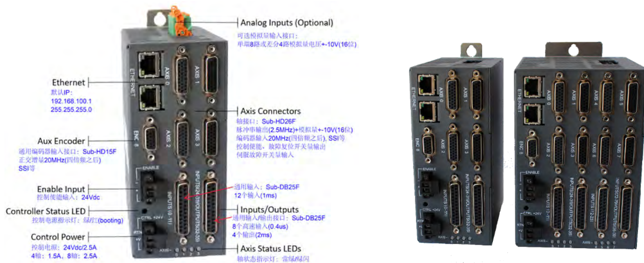
Figure 5 - ACR74C Connectors ACR74C: 4轴Axis0-3+2个通用输入/输出+Enc8 ACR78C: 8轴Axis0-7+4个通用输入/输出+Enc8
